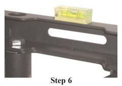
With the help of an assistant, place a level on the center of the mounting rail and level the mount. Mark and drill the second mounting hole.
